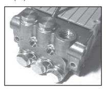
7. Carefully slide the valve casing (#26) out over the plungers with a screwdriver placed between the valve casing and crankcase.
