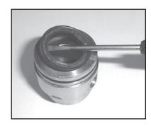
10. Remove the weep grooved seals (23A) from the seal case (#20). Remove the pressure rings (#24).
