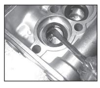
9. Remove the pressure rings (#24) and grooved seals (#23) from the valve casing (#26). Inspect parts for wear and replace if necessary.
